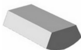
Combination die blanks for making hexagonal nuts
